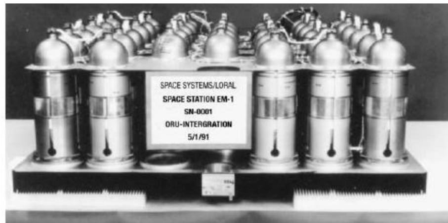
FIGURE 32.8 International Space Station 81-Ah Ni-H 2 38-cell assembly.
