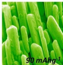
Comparison of \text{LiFePO}_4 nanoplates with thick plates [Saravanan et al. J. Mater. Chem. , 19 (2009) 605].
