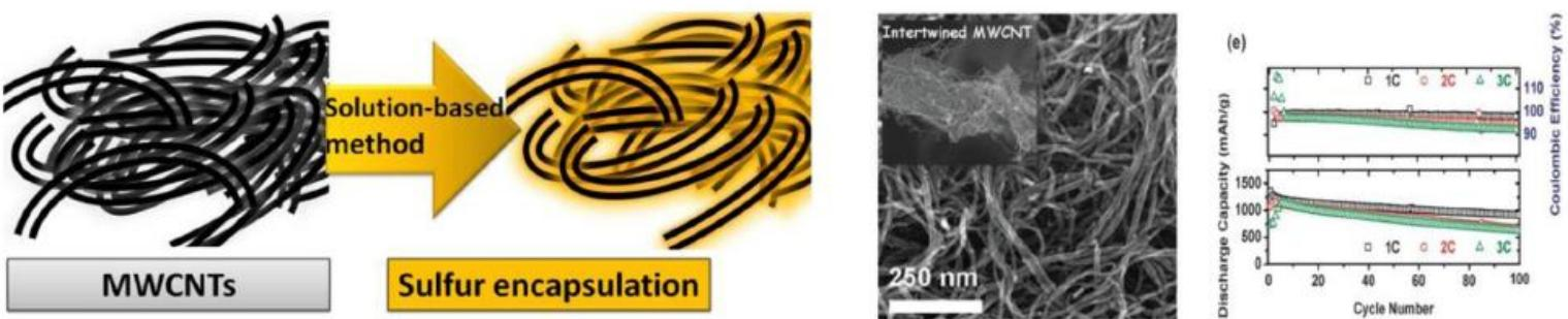
Figure 12. Schematic models, SEM observation (the SEM image of the carbon host is also shown), and cell performance of a representative S–CNT composite. Reprinted with permission from ref 24b. Copyright 2012 The Royal Society of Chemistry.
