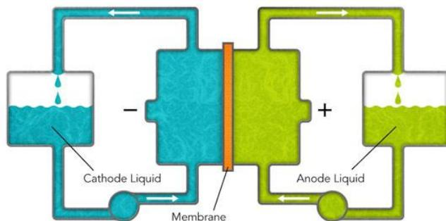
New Lithium-Polysulfide Flow Battery Design
