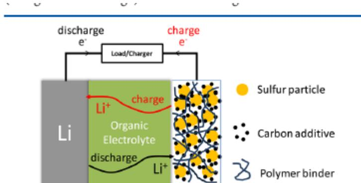
Figure 1. Schematic diagram of a Li-S cell with its charge/discharge operations.
